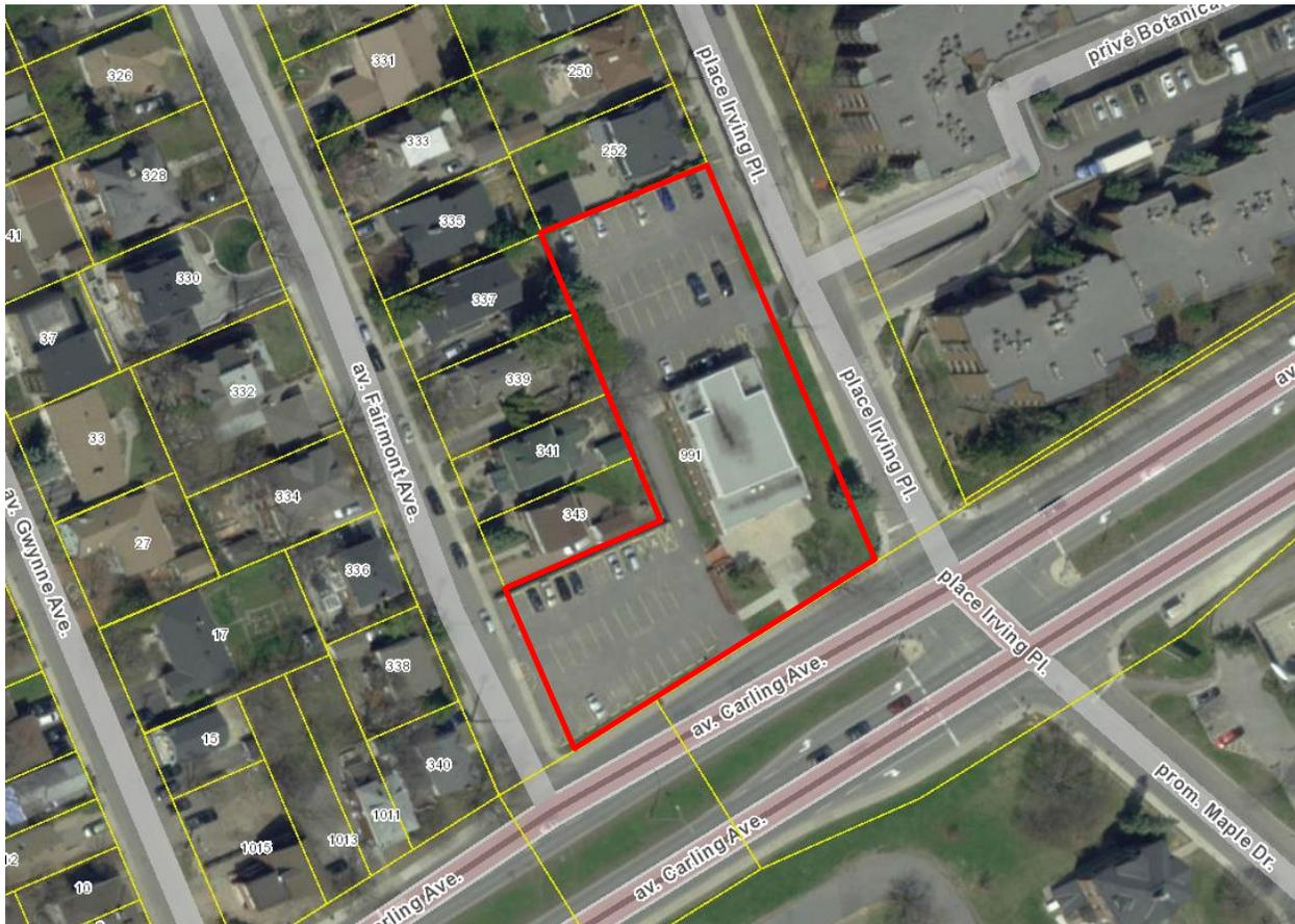
There are 77 parking spaces on the site, of which 3 are barrier-free, though it appears they do not meet the required standard width for a barrier-free parking space. About half of the spaces are located north of the existing building and accessible from Irving Place, and the other half are located west of the existing building and accessible from Fairmont Avenue.
